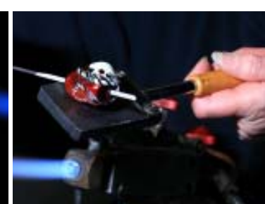
15. Shaping bead with graphite paddle.
