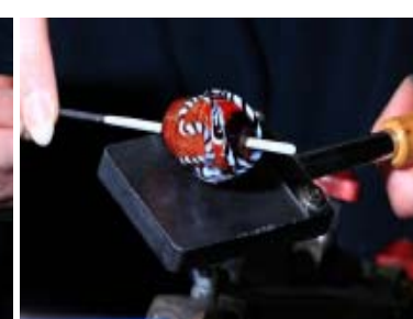
16. Final bead shaping then get bead really hot and molten
