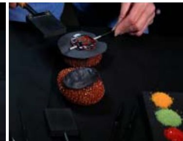
19. Quickly remove the graphite paddle used to press glass or it will chill the glass
