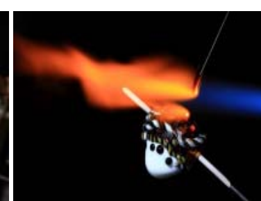
14. Using flame to cut glass from rod.
