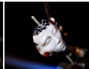
22. Place finished bead into annealing kiln.
