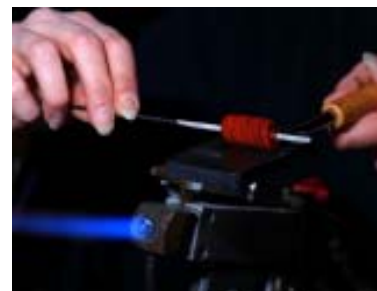
8. Shaping molten glass bead
