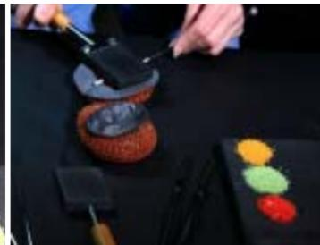
18. Press molten glass into mold.
