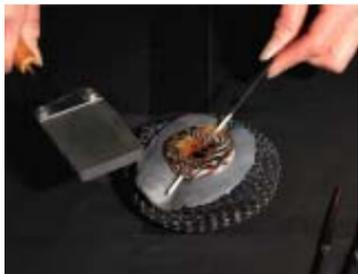
20. Give a light tap to the mold and pull the bead out of the mold
