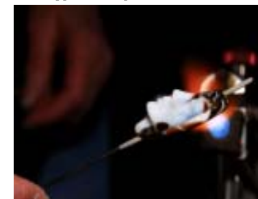
21. Fire-polish any chill marks caused by graphite paddle. Keep face out of flame. Mold Mix 6 does not cause chilling, so there is no need to fire-polish face.
