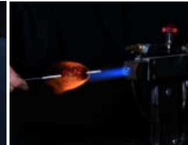
10. Melting frit in flame.
