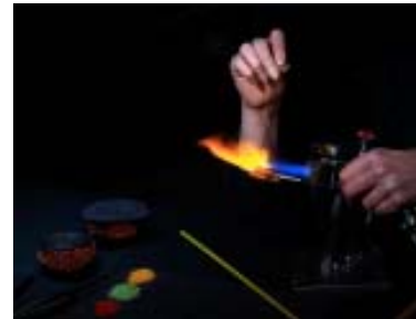
5. Build up molten glass around mandrel that has been dipped in bead release.
