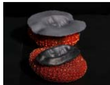
4. Molds sprayed with dry graphite and placed on copper scrub pads to cushion mold while pressing molten glass into it.
