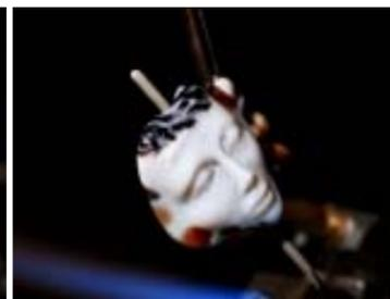
22. Place finished bead into annealing kiln.
